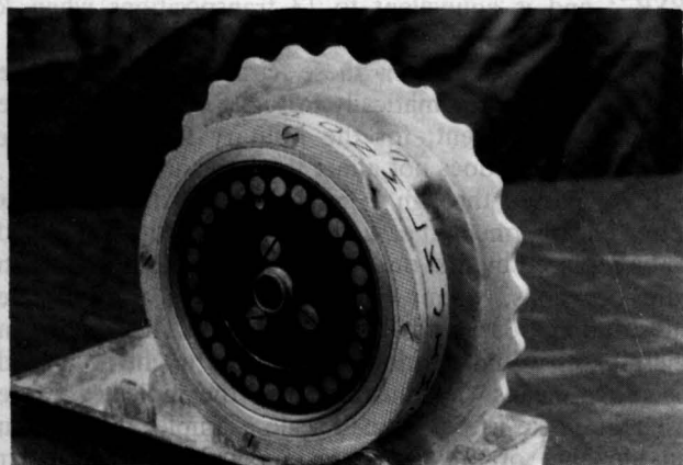
Fig. 4. One of the rotors. Note the notch in the ring at position M
