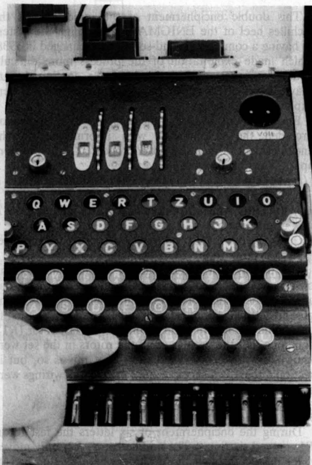
Fig. 3. The ENIGMA ready for use. The rotors are set at AAB, the letter C has just been enciphered and the cipher letter J has lit up
